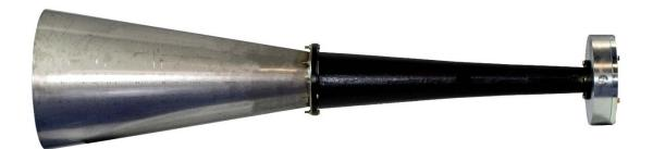
ACS acoustic cleaners use compressed air to flex a titanium diaphragm to produce pressure pulses that are amplified by the bell. The resulting low frequency/high energy sound waves that are emitted resonates/dislodges particulate deposits. The displaced particulate deposits are then removed by gravity and/or gas flow.
